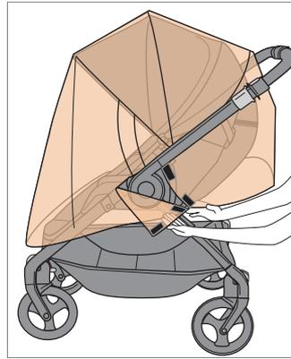
Guide the flap attached to the front of the weather shield toward the back seat pocket and fasten the two velcro strips. Do this for both sides.
