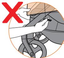
Do not wrap the velcro around the angled leg tube.
