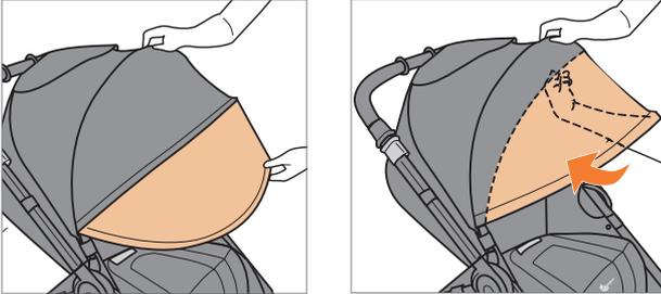
Pull the sunshade all the way forward and tuck the sunshade extension under as far as it will go. The front edge of the sunshade should be taut with no loose fabric drooping down.
